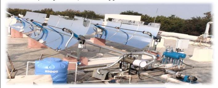
• The parabolic-trough test rig facility has features for simultaneous testing of standard and indigenous solar receiver tubes. It has a thermic fluid-based closed-loop system which can operate between 50 to 350°C temperature range. It can conduct heat gain studies in real-field conditions with the actual measurement of solar irradiance condition and has an electrical heater support for measuring the actual heat loss of solar receivers at different operating temperatures.
